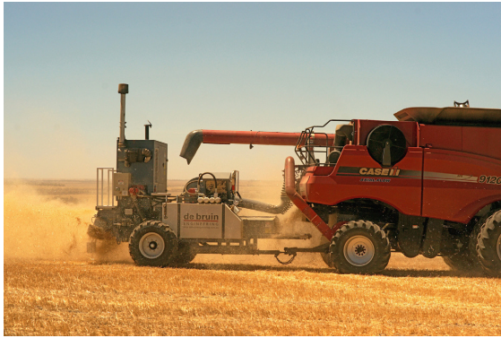
FIG. 5. A “seed destructor” attached to the back end of a combine harvester in an Australian grain field. The machine grinds and destroys weed seeds contained in crop residue passing through the combine. Photo courtesy of J. Millhouse.
